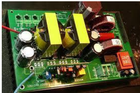
Fig. 2.1: Inverter inner circuitry.
