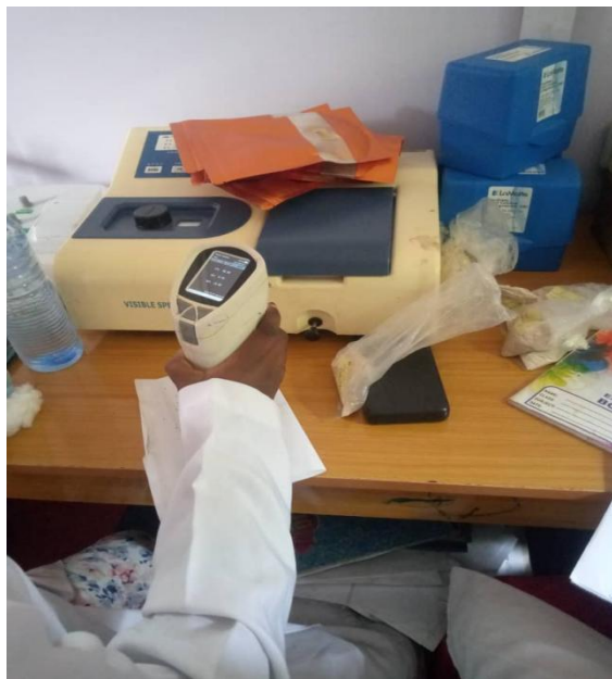
Plate 3.3 Presenting the Determination of the Colorimetre of the okro
