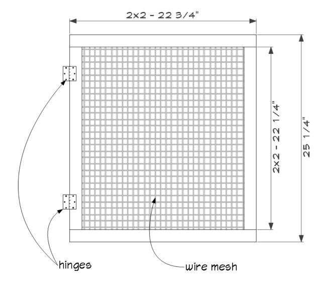
The door as shown was assembled using exterior wood glue and 2 1/2" pocket hole screws. Cut the wire mesh to size and attach to the door frame using 18 gauge 3/4" galvanized staples.
