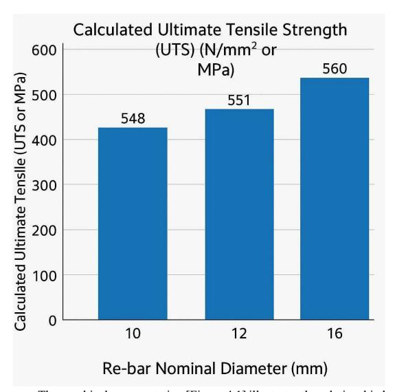
The graphical representation [Figure 4.1] illustrates the relationship between rebar diameter and Ultimate Tensile Strength. It was observed that while the 12mm and 16mm re-bars consistently met and slightly exceeded the standard, the 10mm rebar exhibited a slightly lower UTS. Despite this, the UTS values across the tested diameters (548, 551, and 560 N/mm²) are relatively close, suggesting a general consistency in material properties, albeit with a slight dip for the 10mm sample.
