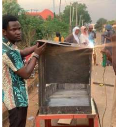
Figure 3.3.2 welded framework of the indirect solar dryer
