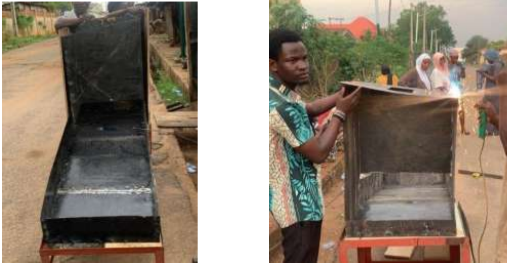
Figure 3.3.2 welded framework of the indirect solar dryer
