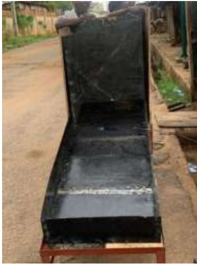
Figure 3.3.2 welded framework of the indirect solar dryer
