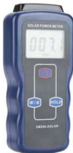
Figure 3.2.3 Solar Radiation Meter (Pyranometer)
