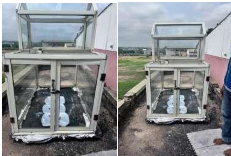
Figure 3.3.4 Complete construction of the greenhouse solar dryer
