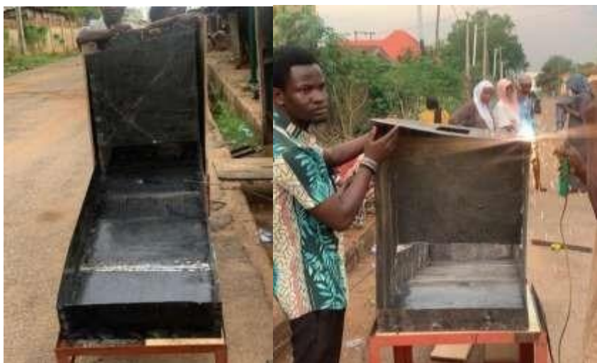
Figure 3.3.2 welded framework of the indirect solar dryer
