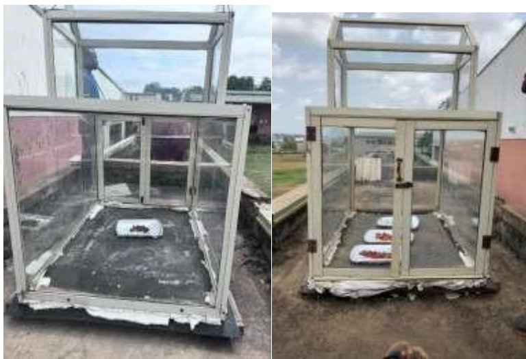
Figure 3.3.4 completed construction of the greenhouse solar dryer
