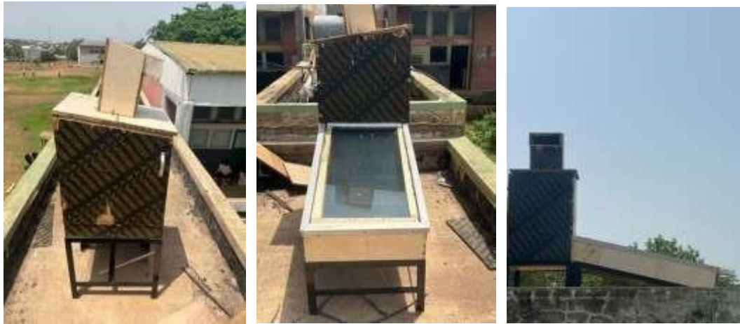
Figure 3.3.3 completed construction of the indirect solar dryer
