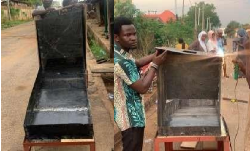
Figure 3.3.2 welded framework of the indirect solar dryer
