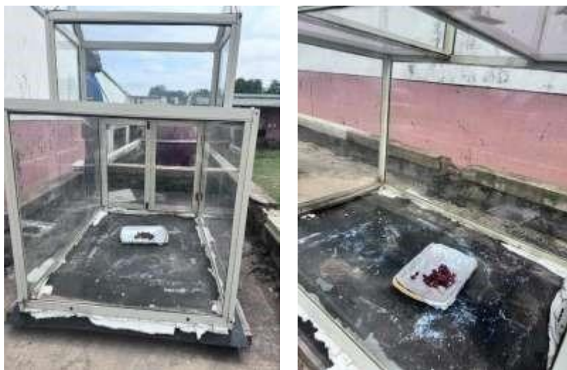
Figure 3.4.2: Tray placed inside Greenhouse Solar Dryer
