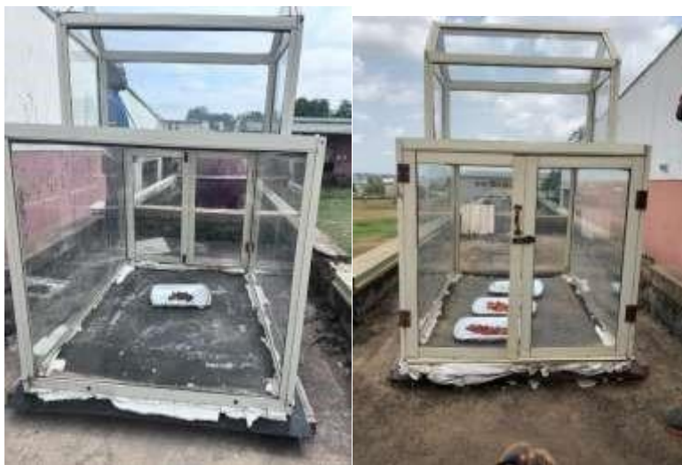
Figure 3.3.4 completed construction of the greenhouse solar dryer
