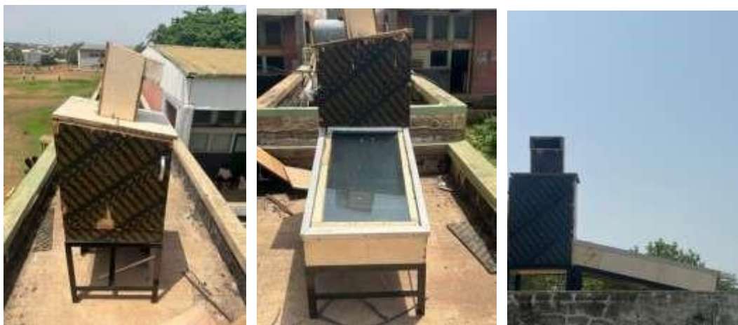
Figure 3.3.3 completed construction of the indirect solar dryer
