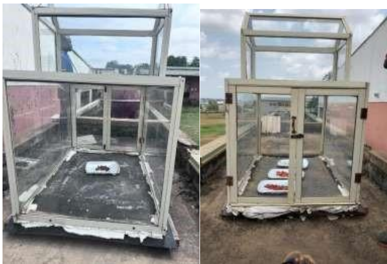
Figure 3.3.4 completed construction of the greenhouse solar dryer
