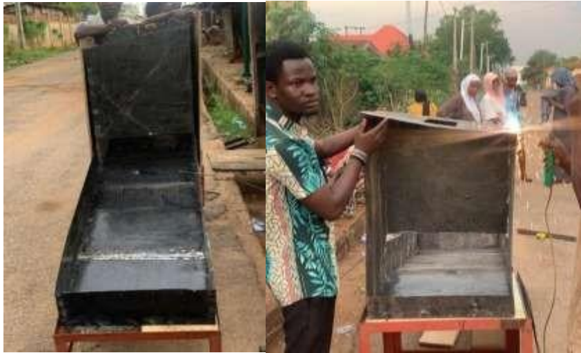
Figure 3.3.2 welded framework of the indirect solar dryer
