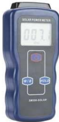
Figure 3.2.3 Solar Radiation Meter (Pyranometer)
