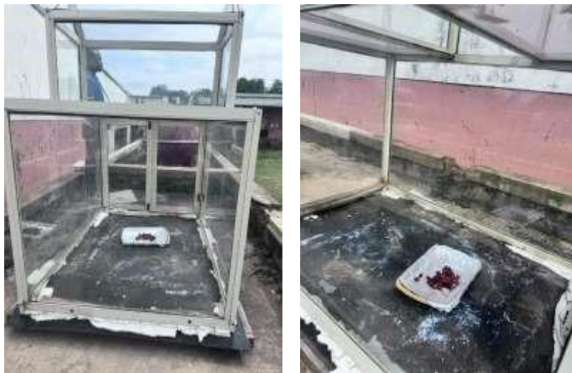
Figure 3.4.2: Tray placed inside Greenhouse Solar Dryer
