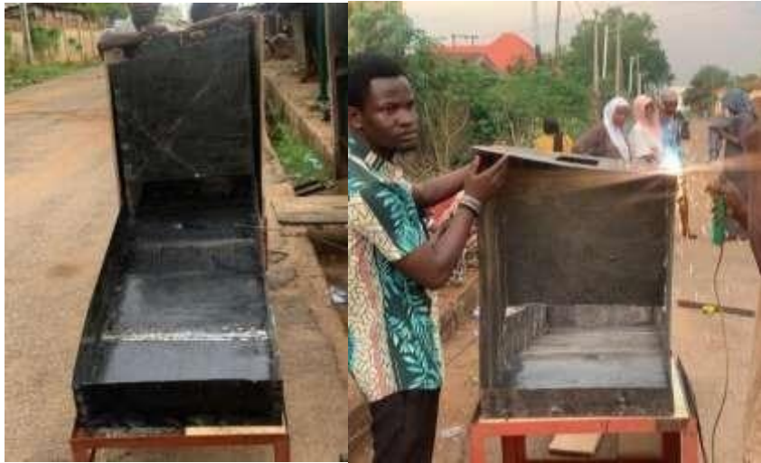
Figure 3.3.2 welded framework of the indirect solar dryer
