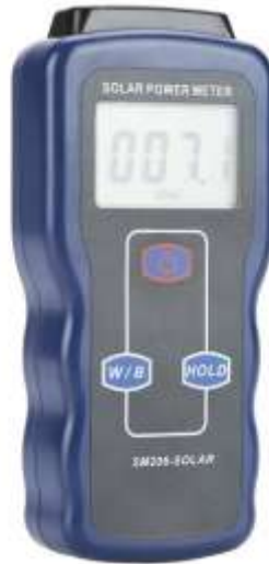
Figure 3.2.3 Solar Radiation Meter (Pyranometer)
