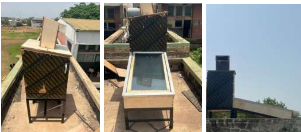
Figure 3.3.3 completed construction of the indirect solar dryer
