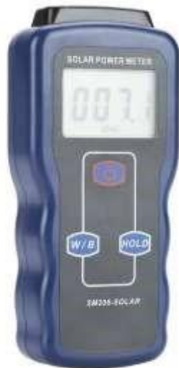
Figure 3.2.3 Solar Radiation Meter (Pyranometer)
