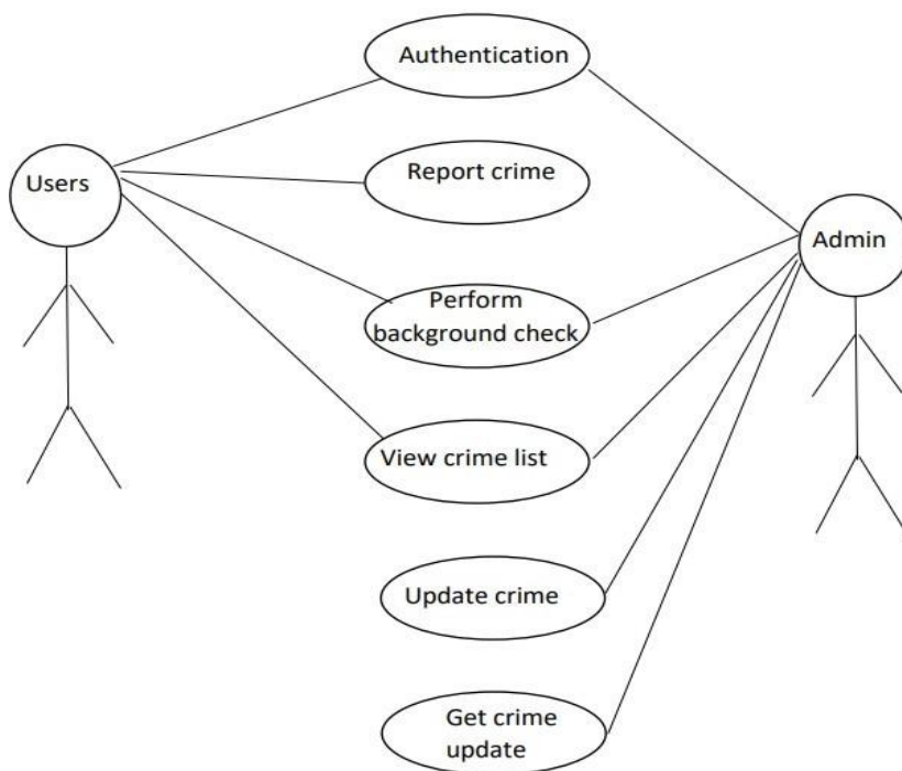
Fig 4: Use Case Diagram
