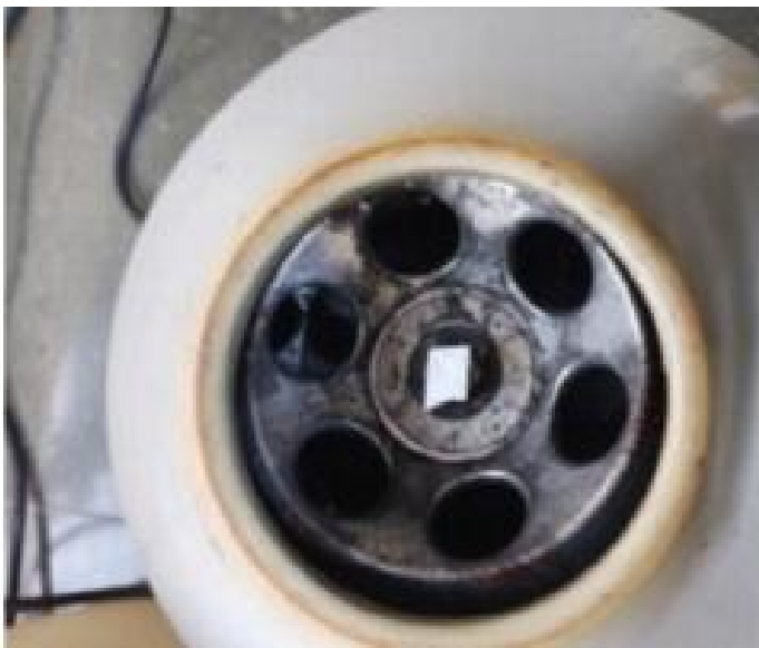
Figure 15: We measure the Torque RPM of no load using a tachometer which takes place in Bahmed Clinical/diagnostic Ltd.
