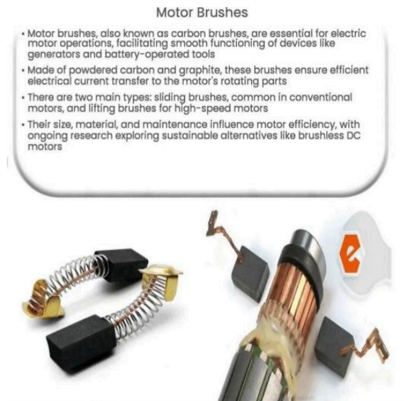
Figure 6: A Pictorial diagram of DC Motor Brushes.
