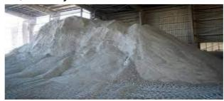
Gypsum plays an important role in cement production, it controls the setting time of cement, and that is, it slows down the hydration process in cement once it is mixed with water. The effects of gyp sum on cement are as follows:
