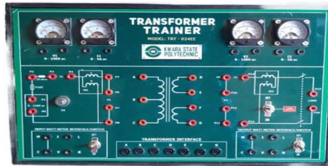
Figure3.6:Front view of a Single Phase Trainer
