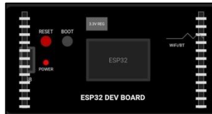
Figure 2.2: ESP32 Development Board Layout
