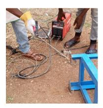
• Gas metal are welding: Commonly termed MIG (metal, inert gas), uses a wire feeding gun that feed wire at an adjustable speed and flows an argon-based shielding gas and carbon dioxide (Coz) over the weld puddle to protect it from atmospheric contamination.
