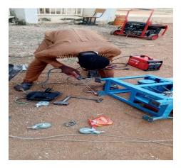
• Shielded metal are welding: Also known as "stick welding", uses an electrode that has lux, the protectant for the puddle, around it. The electrode holder holds the electrode as it slowly melt away.
