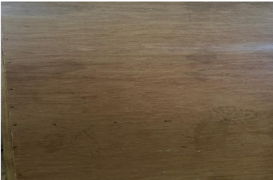
Plate 3.2: Plywood for suspended floor
