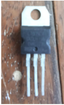
Fig 3.8: IMAGE OF A VOLTAGE REGULATOR
