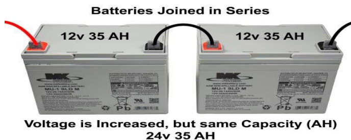
Fig 3.1 showing Battery (24V Battery)
