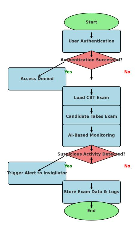
Figure 3.5 Flowchart Diagram for Smart Solar CBT Examination Monitoring System.
