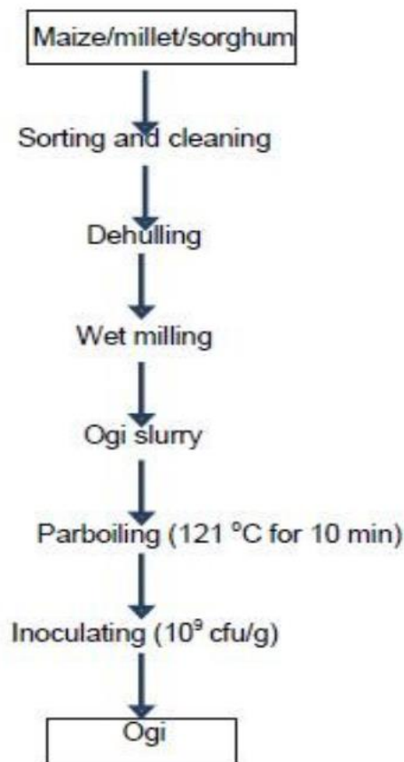
Fig. 4: Preparation of ogi in a controlled environment
