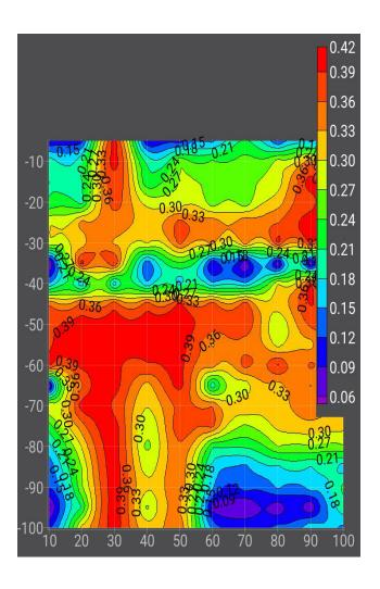
Figure 4.3:2D Resistivity Tomogram of Profile C-C'
