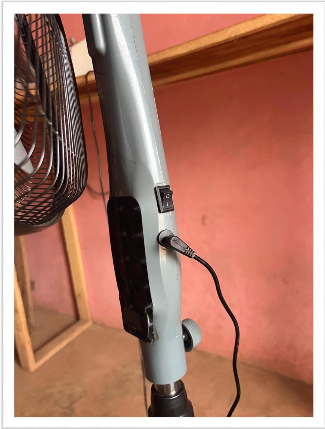
Fig 4.1.4: Showing the input, manual and the automatic switch of the smart fan
