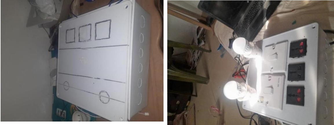
Figure13 The Home Automation System Casing
