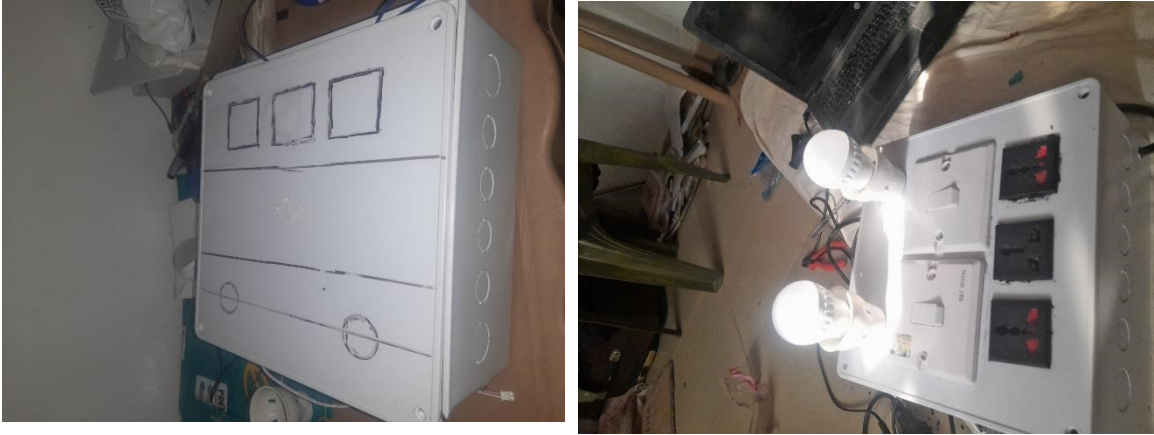
Figure13 The Home Automation System Casing
