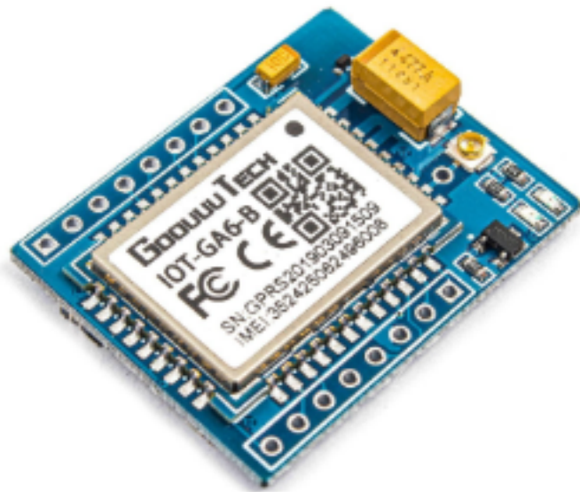
Figure 4.4: GSM or Wi-Fi Module
