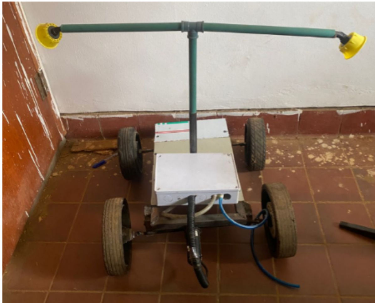
Figure 4.1: Wireless Smart Irrigation System
