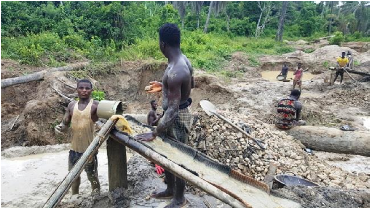
Plates 3.1: Typical Artisanal Small-Scale Gold Mining Process in the Study Area using a Sluice Box
