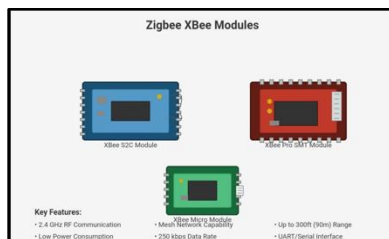
Figure 2.7: Zigbee XBee Modules and Key Features.
