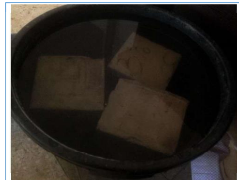
Fig 3.2: Curing of the cubes
