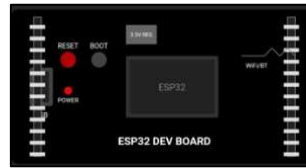
Figure 2.2: ESP32 Development Board Layout
