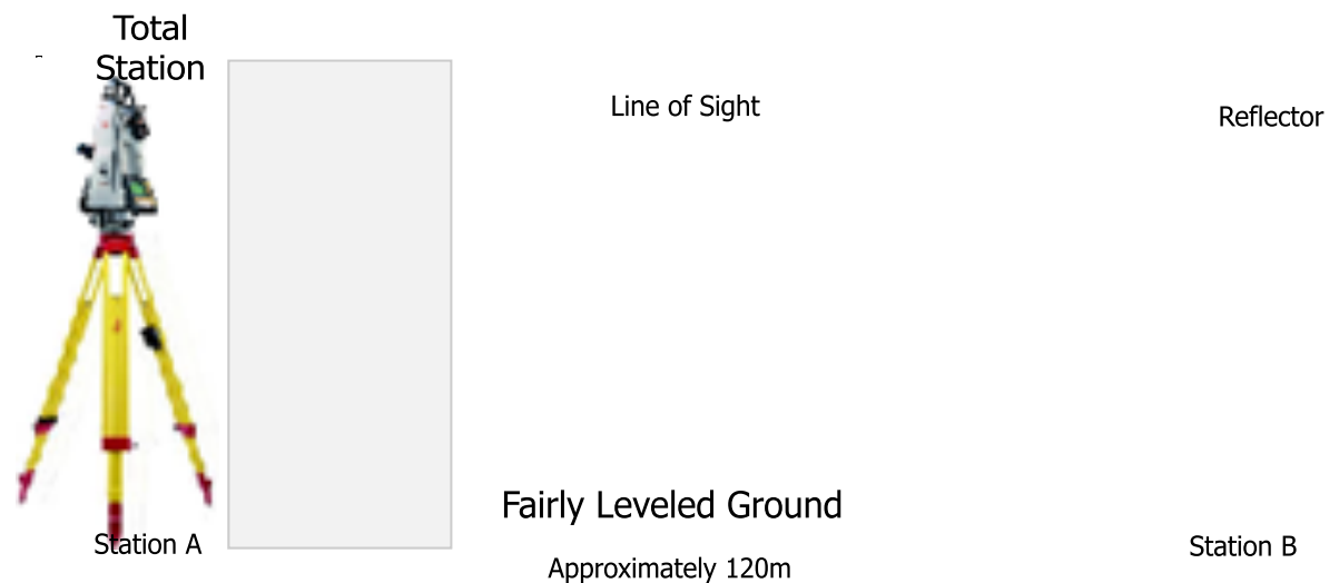
Figure 1.6. : Instrument set-up for horizontal collimation test and vertical index test
