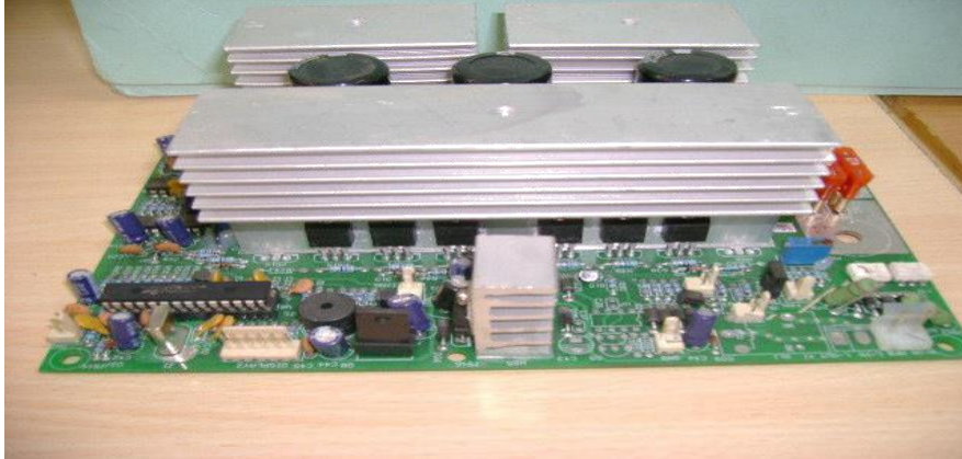
Fig. 2.1: Inverter inner circuitry.
