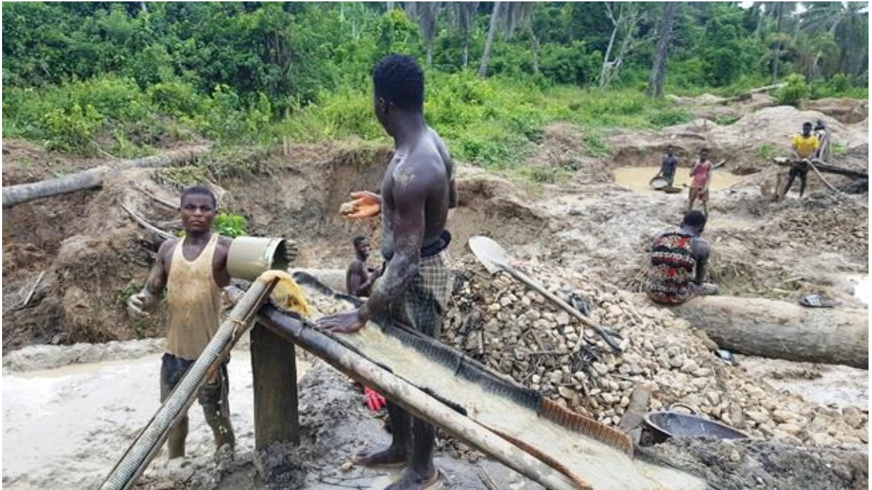
Plate 3.1: Typical Artisanal Small-Scale Gold Mining Process in the Study Area using a Sluice Box
