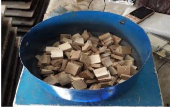
Fig. 3.1: Processed Bamboo Chips Used as Partial Coarse Aggregate Replacement
