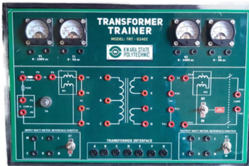
Figure3.6:Front view of a Single Phase Trainer
