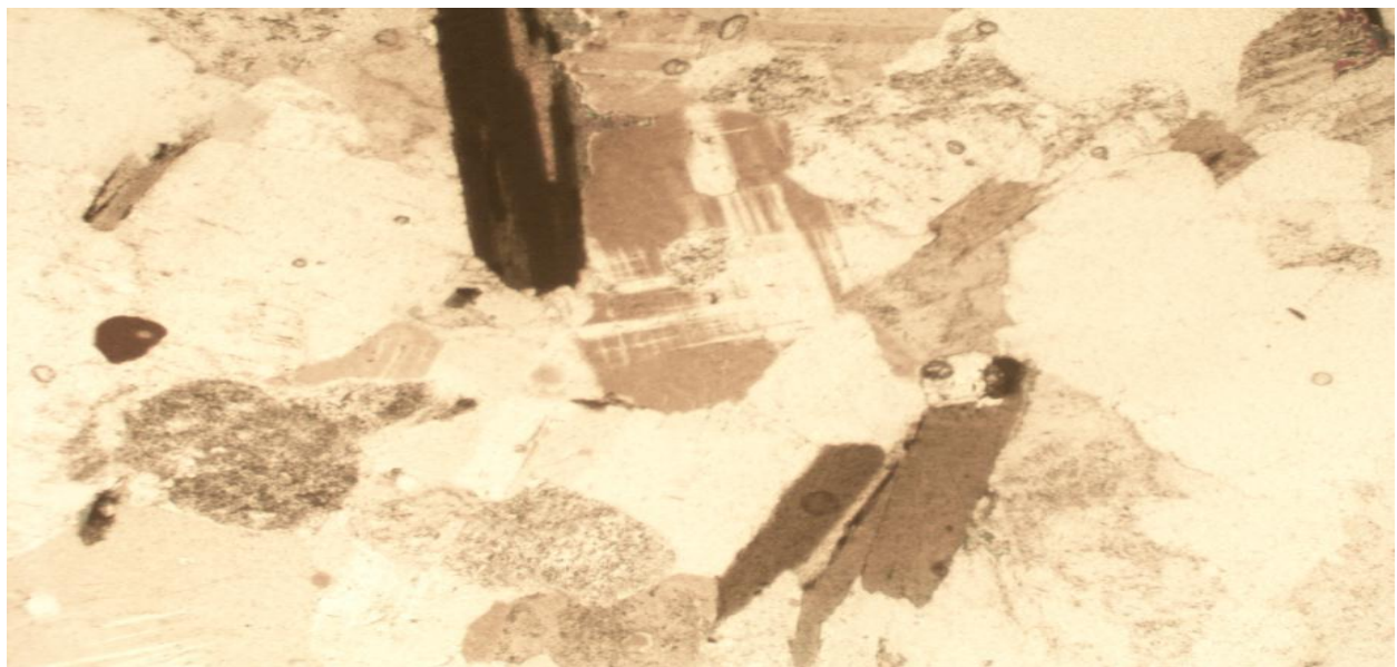
Plate 4.5: Photomicrograph of migmatite gneiss under Plane Polarized Light (PPL) showing the various shades of colours of mineral grains, Quartz (Q), Biotite (B), Plagioclase feldspar.
