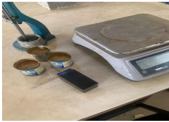
Figure 3.5: Sand Samples in Can for Moisture Content Test
