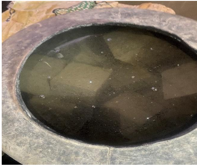
Figure 3.11: Curing of Cubes
