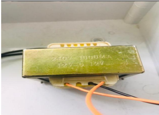
Figure 3.4: 240V/12V Step-Down Transformer
