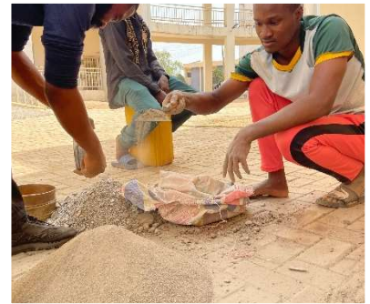
fig 3.7 : Sieving of Stone dust
