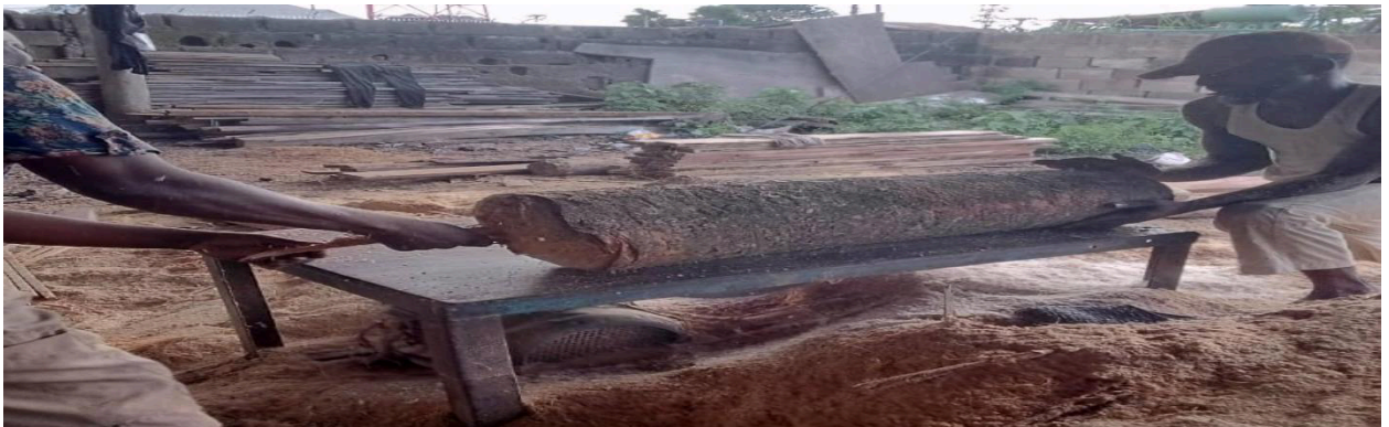
Plate I: Sawing of timber from the log at the sawmill
