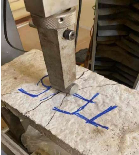
Plate V: Arrangement and Failure Mode of Timber Reinforced Slab
