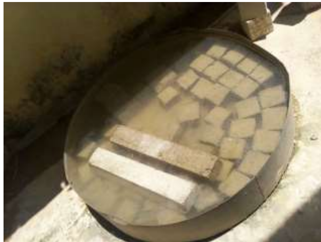
Plate 7: Curing of the beam produced from calcium chloride admixture
