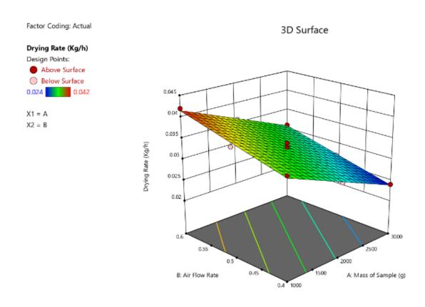
Fig 4.1: Effect of Air Flow Rate and Mass of Sample on the Drying Rate of Cocoa
