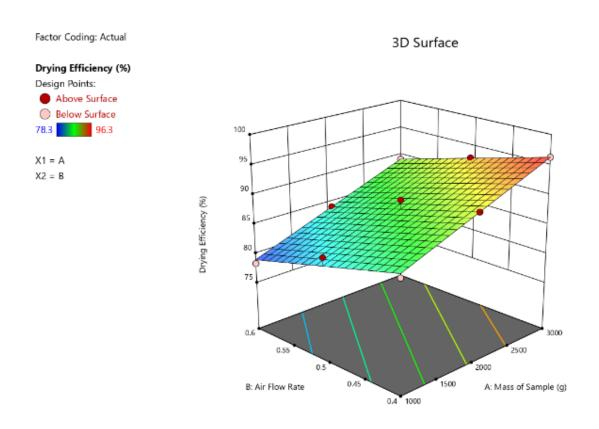
Fig 4.2: Effect of Air Flow Rate and Mass of Sample on the Drying Efficiency of Cocoa
